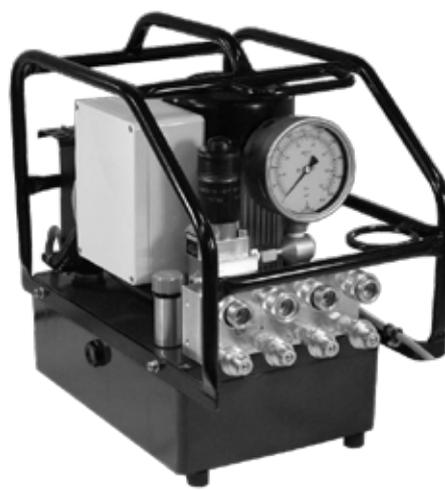
3-stage electro-hydraulic unit for operation of hydraulic torque tools; Extremely compact build, 2-button safety remote control with 5 metres long connection cable with plug-in system; Available for alternating voltages from 100-230 Volt 50/60 Hz with a maximum pressure up to 800 bar (optionally 700 bar); Simple and precise pressure or torque setting
