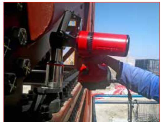
Right Angle Gearbox fitted to EvoTorque®2
